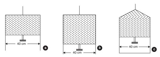
**Ans.** (*a*) Here, length of the film supporting the weight = 40 cm = 0.4 m. Total weight supported (or force) =  $4.5 \times 10^{-2}$  N.
