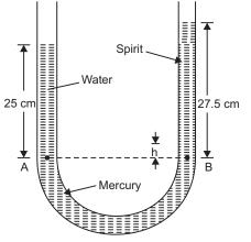
Mercury will rise in the arm containing spirit; the difference in levels of mercury will be 0.2206 cm.
