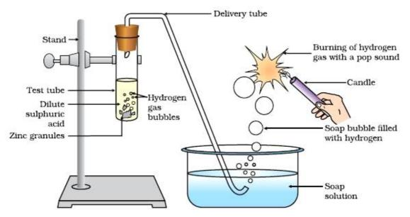
Take few pieces of zinc granules and add 5 ml of dilute H2SO4. Shake it and pass the gas produced into a soap solution. The bubbles of the soap solution are formed. These soap bubbles contain hydrogen gas.
