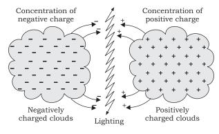
A cloud has the negative charges concentrated at the base and positive charges concentrated at the upper region. When a charged cloud passes over a tall building or a tall tree, it induces an opposite charge on them. The negative charge at the base of the clouds pull the positive charges induced on the tall buildings upwards at a tremendous speed. As soon as the negative and positive charges
