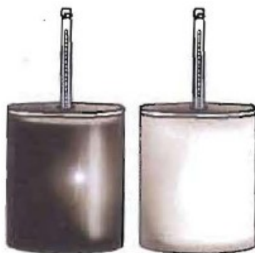
Absorption of radiant heat by black and white cans
